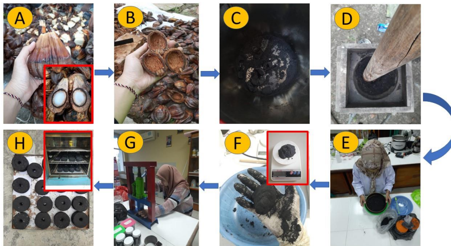
Figure 3. The process of making charcoal briquettes from nipah fruit fiber and shell. A. Fruit cutting, B. Separation of fruit flesh from fibers and shells, C. Carbonization of fibers and shells, D. Refining of carbonized charcoal, E. sifting of charcoal, F. Mixing charcoal with adhesives, G. Molding of briquettes, H. Products molded charcoal briquettes.
